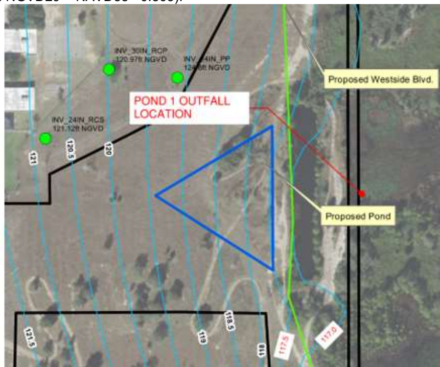
Figure 2: Snippet of Royal Consulting Services, Inc./Toho Water Authority's Model Predicted Groundwater Elevation at the end of the wet season with the outfall location denoted.
